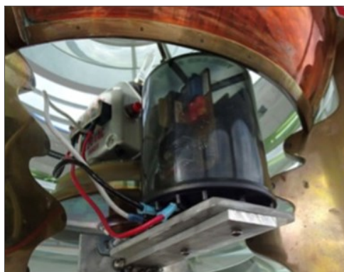
Figure B. Plastic Cylinder Holding Circuit Board.
